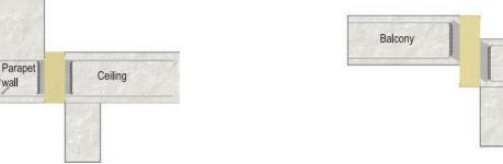
KP-900 connector, used at support joints of the balcony slab with the ceiling slab - transfer of  $V_{\mbox{\scriptsize Rd}}$  shear forces (±). Reinforcement bars of stainless steel.
