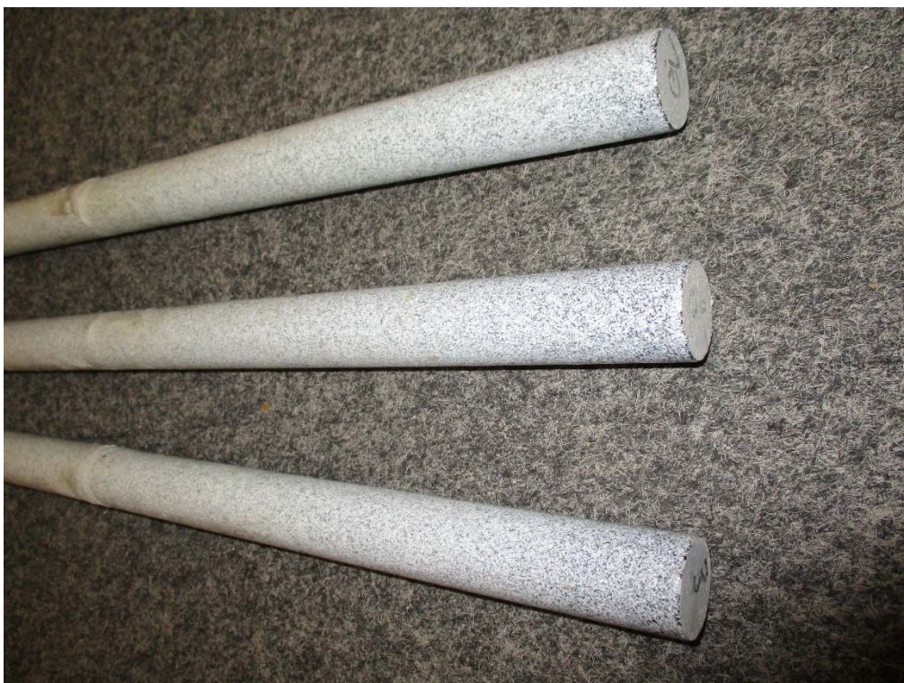
Picture 2: View of opposite side of lateral surface of dowels after test execution without damage of coating.
