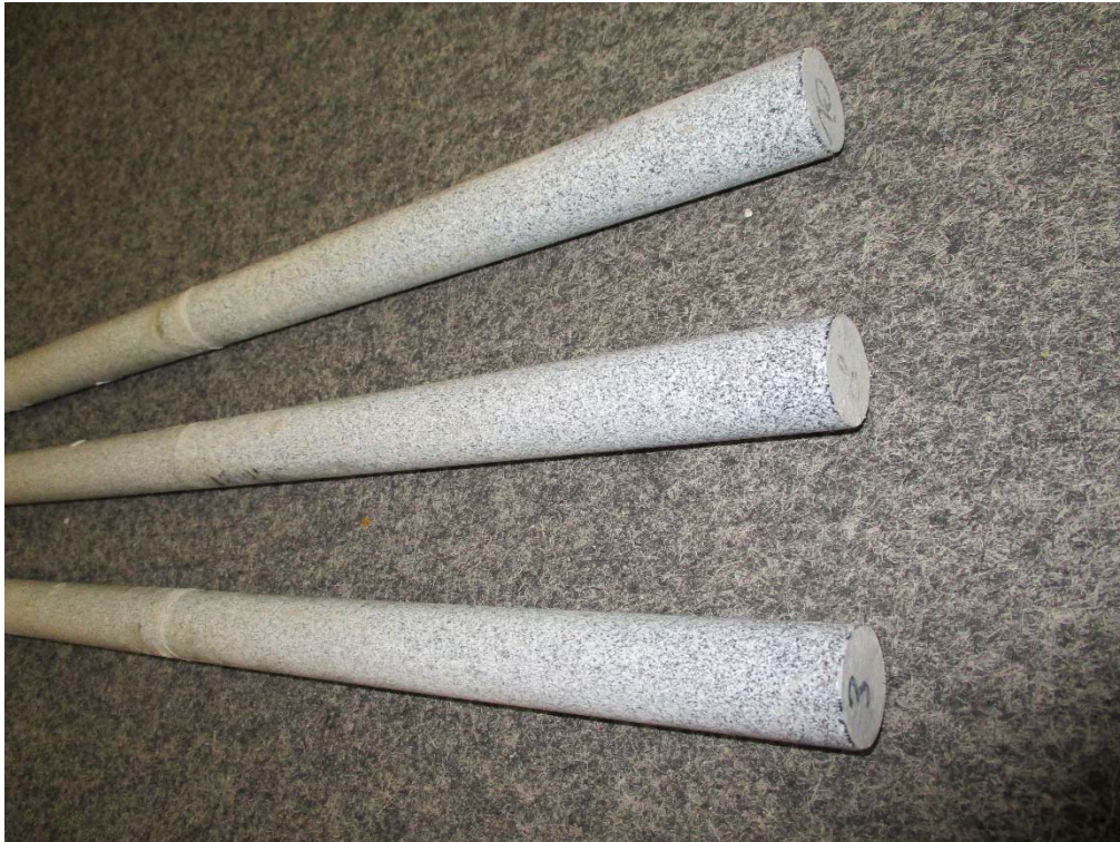
Picture 1: Tested dowels No.3, 8 and 10 without damage or delamination of coating.
