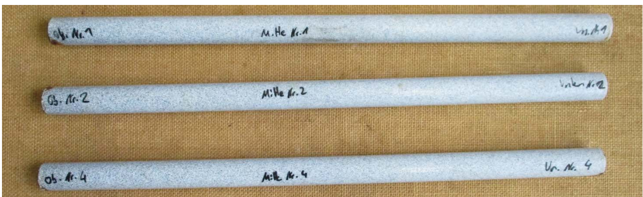
Picture 3: Plastic coated surface of dowels does not show any rust in regarded area of lateral surface after 240 hours at neural salt-spray.
