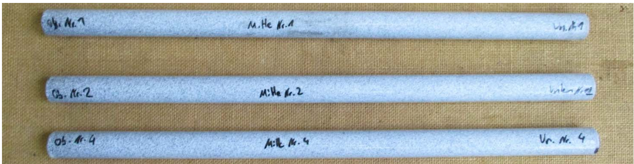
Picture 1: Plastic coated surface of investigated dowels before corrosion testing.
