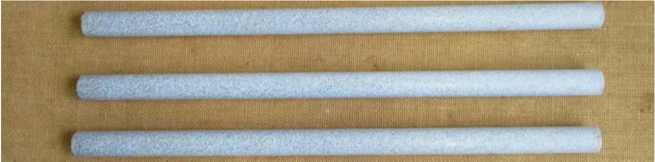
Picture 4: Opposite plastic coated surface of dowels without any rust in regarded area of lateral surface after 240 hours at neutral salt-spray.
