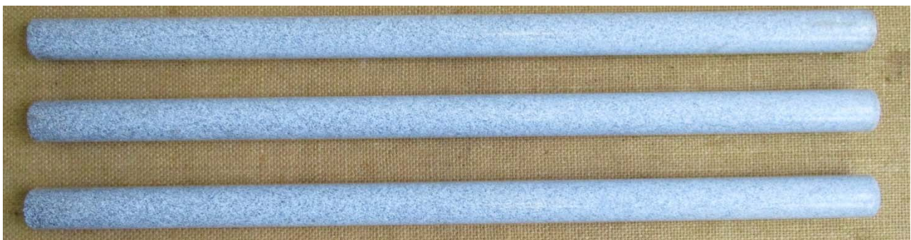
Picture 2: Opposite surface of investigated dowels before corrosion testing.
