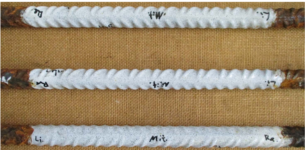
Picture 7: View of plastic coated area of tie bars after 240 hours salt-spray. No rust was observed in regarded area of lateral surface (200 mm in centre of tie bar).
